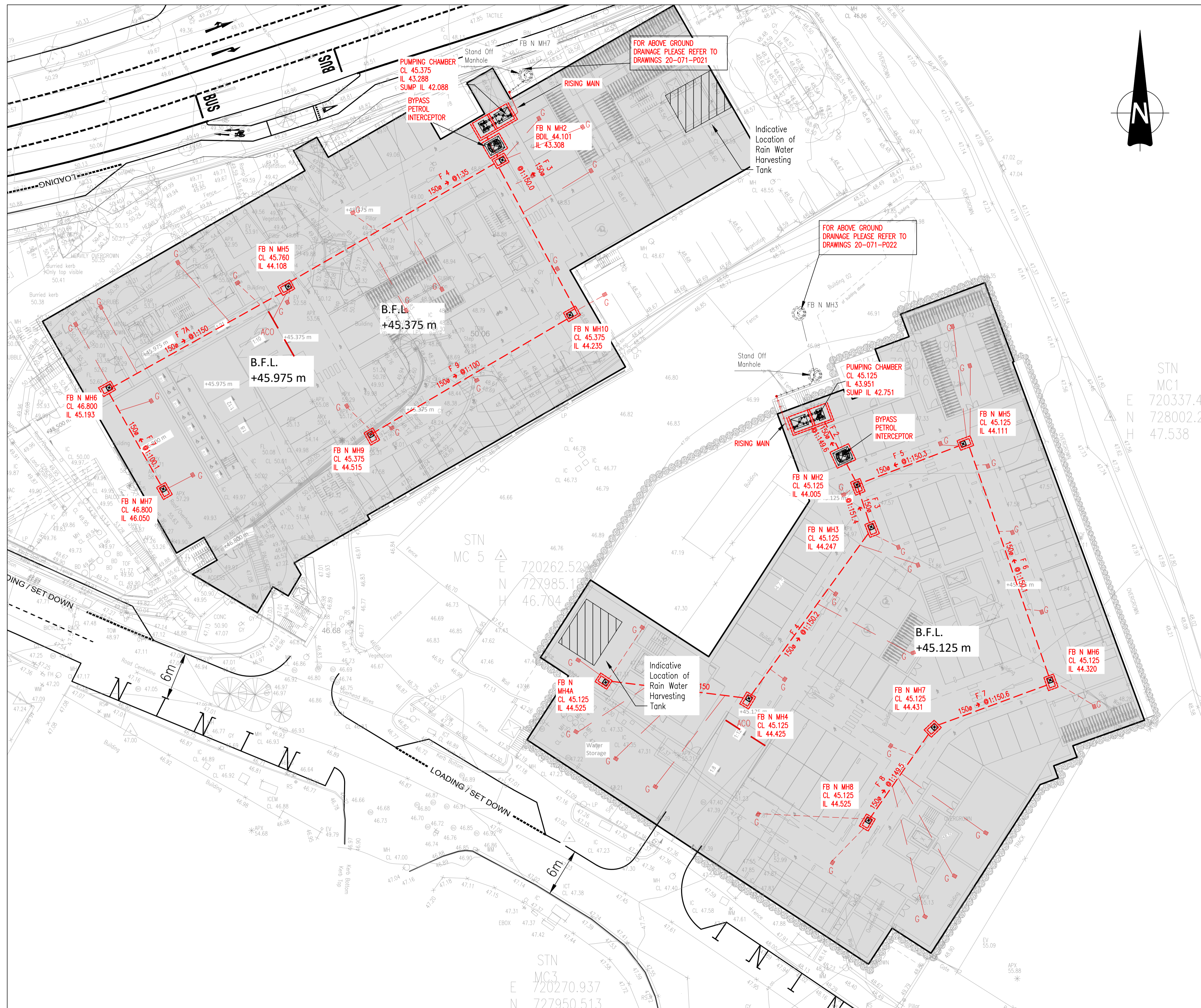
PLAN VIEW PROPOSED BASEMENT DRAINAGE LAYOUT SCALE 1:250 @A1
