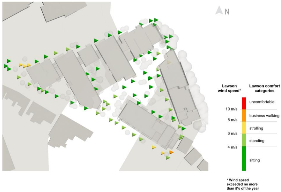
Figure 21: Lawson wind speeds at key locations along the thoroughfares (existing surroundings with landscaping)
