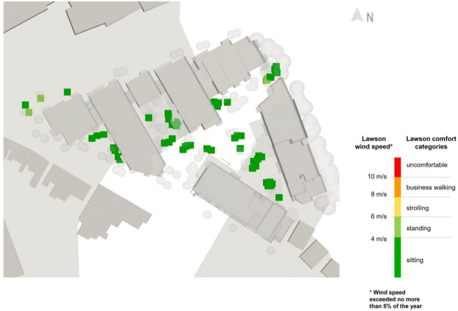
Figure 32: Lawson wind speeds in key locations at the public seating spaces (cumulative surroundings with landscaping)
