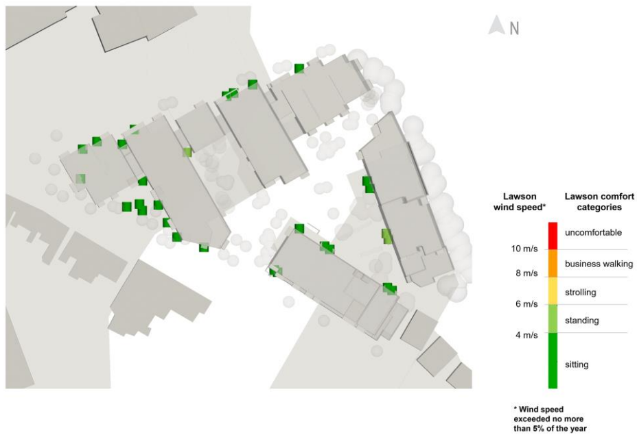
Figure 23: Lawson wind speeds at the primary entrances (existing surroundings with landscaping)
