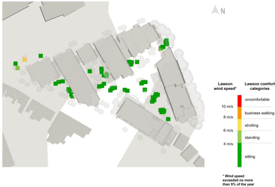
Figure 25: Lawson wind speeds at key locations of the public seating spaces (existing surroundings with landscaping)
