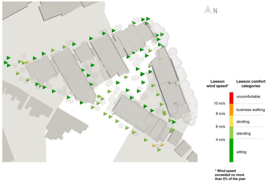
Figure 28: Lawson wind speeds at key locations along the thoroughfares (cumulative surroundings with landscaping)
