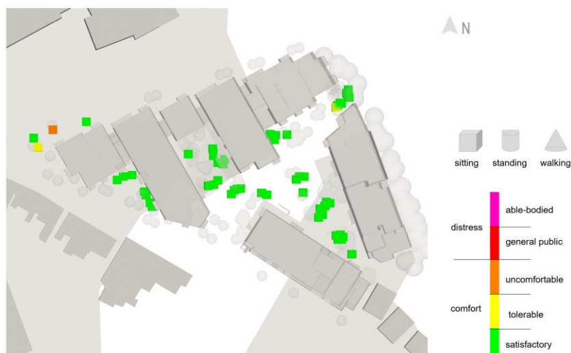
Figure 25: Lawson wind speeds at key locations of the public seating spaces (existing surroundings with landscaping)
