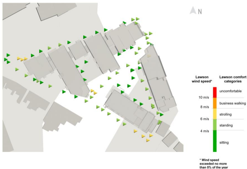
Figure 7. Lawson wind speeds at key locations along the thoroughfares (Baseline)
