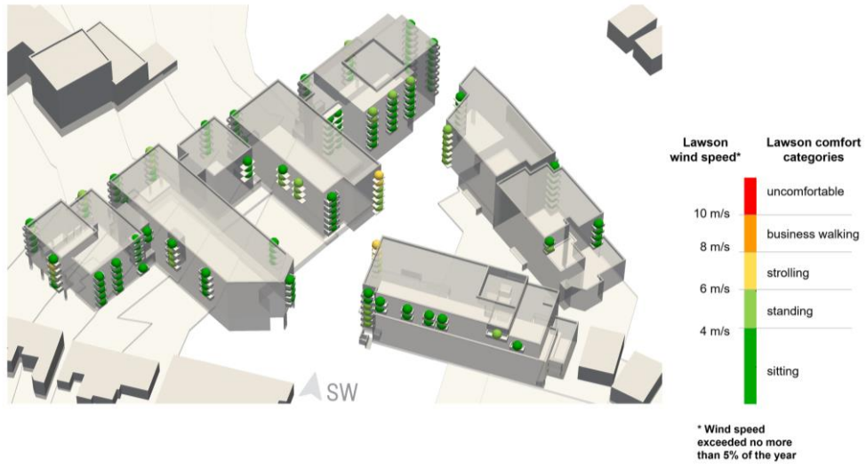
Figure 14: Lawson wind speeds at the balconies (view from southwest)
