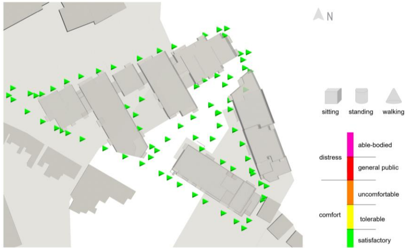
Figure 8. Lawson criteria at key locations along the thoroughfares (Baseline)
