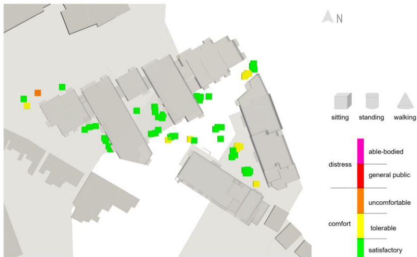
Figure 12. Lawson criteria at key locations of the public seating spaces (Baseline)
